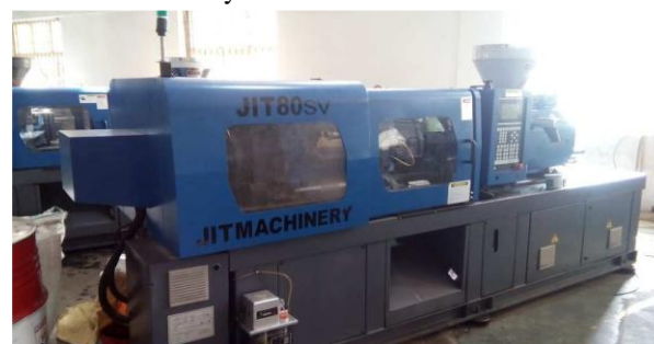
Fig. 4.1: Injection molding machine uses for Experiment (CIPET)
