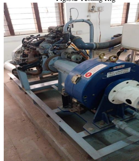
Fig 3.3 Break Torque Measuring system
