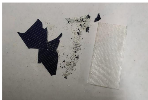
Figure 3.2: Solar cells, Glass, and residual obtained from tube furnace after the experiment
