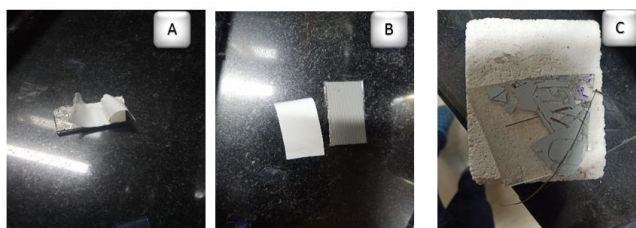
Figure 3.6: Manual separation of intact back sheet/glass, a) Unsuccessful separation of back sheet in hot plate at 45°C, b) Successful separation of back sheet in hot plate at 100°C, c) Separation of glass after pyrolysis at 500°C.
